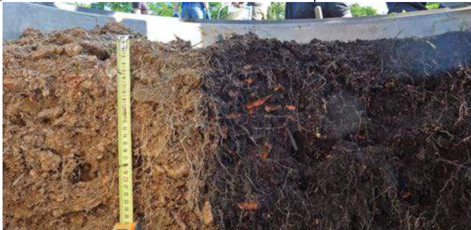
Structural materials: (on the left: excavation subsoil+concrete, on the right greenwaste compost+bricks) © SITERRE project, ADEME, France
